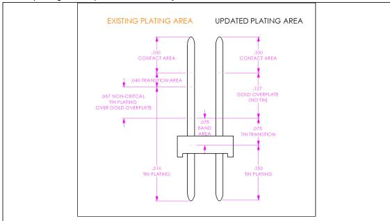
Double row connector shown. The visible tin plated area is lowered closer to the insulator.
